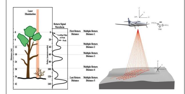
LiDAR system consists with GPS, IMU, Light emitting scanning laser, precise clock and digital camera
