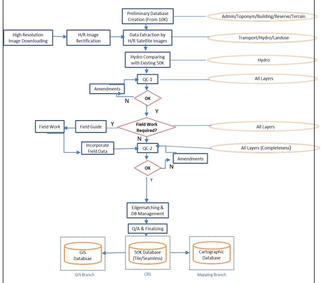
After compiling field data and edge comparison with other sheets, database is finalized. During the finalization process, all data compared with existing 1:10,000 /1:50,000 topographic data, one inch map data, satellite images and all other existing digital data. Therefore, whole process of the creation of database takes 10-12 months for one tile or 1000sqkm.
